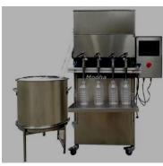
Fig 22: Filling/Bottling Unit for RTS/Juice
