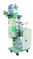
Fig 117: Fill-Seal Machine for Tomato Sauce
