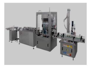
Fig 116: Automatic Paste Filling Machine
