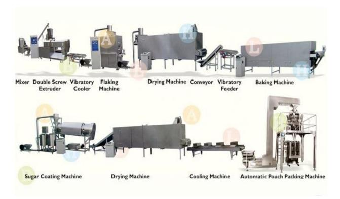
Fig 83: Corn Flakes Processing Line
