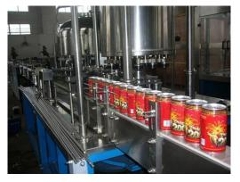
Fig 162: Can Filling Machine
