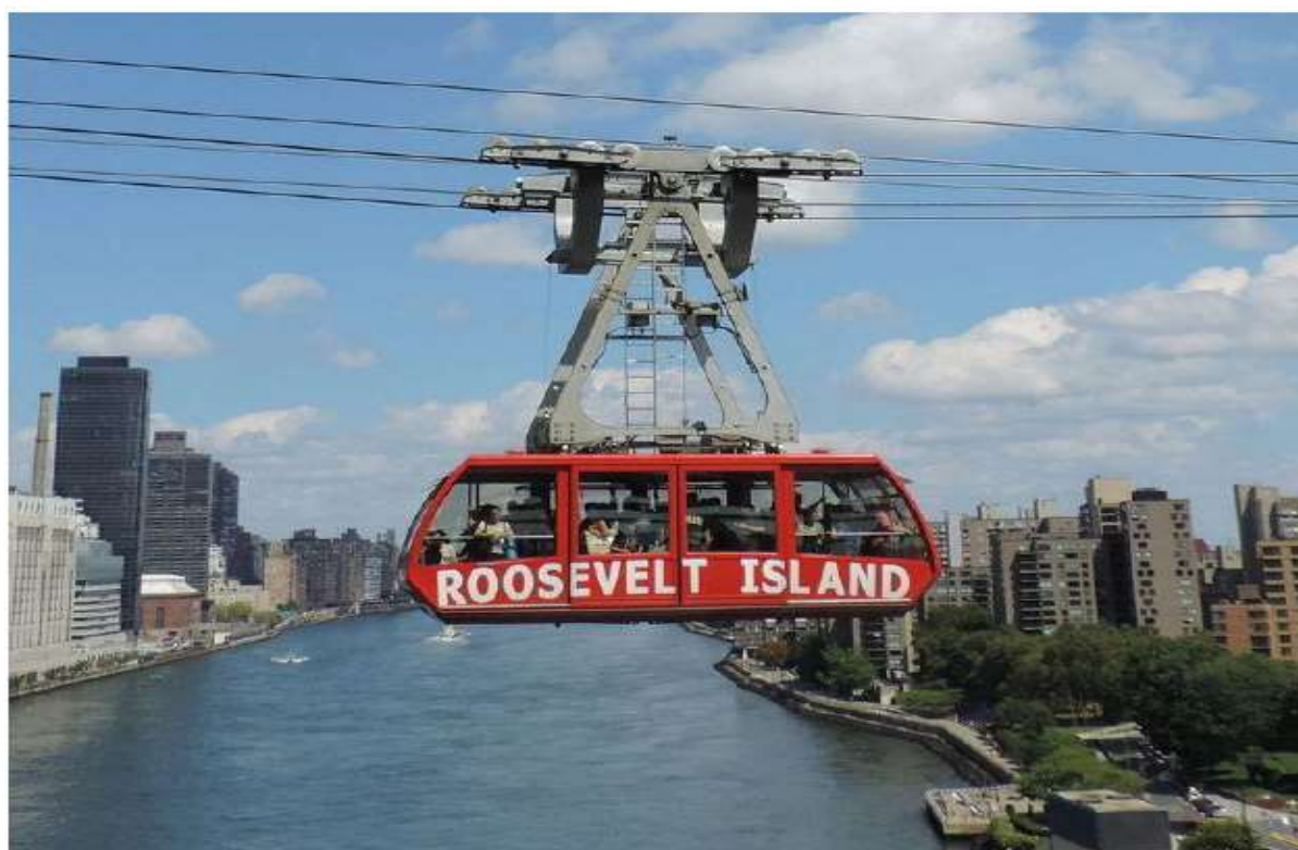
Figure 7-5 Jig Back Ropeway
