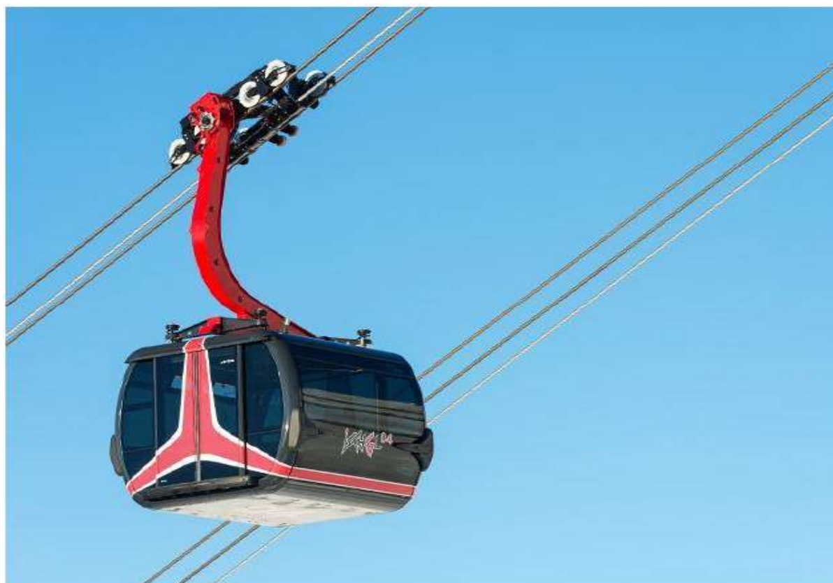
Figure 7-3 Tri Cable Ropeway
